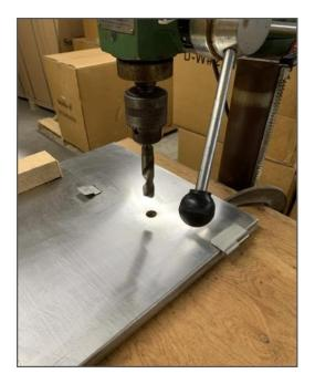
You will need to drill a 3/4" diameter hole on the smoker for the generator smoke tube. We use the door as it is easy to remove from the smoker and it can be setup on a drill press. Make sure you have a sharp drill bit and you need to complete the drilling very slowly. The attached photos are a door for a model 2 or 3 smoker. A 5" up and 5" overlooking left to right hole was drilled. This position will allow enough space to access the door latches.
