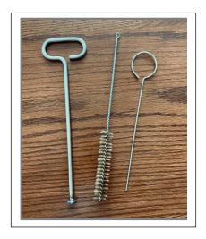
For the best performance when using your generator, clean the main body, smoke tube, and air nipple to remove the buildup of creosote. We recommend using drain cleaner and then thoroughly rinse all the parts with fresh water to remove all chemicals prior to next use. We now offer a cleaning kit for the Bella Smoke Generator.
